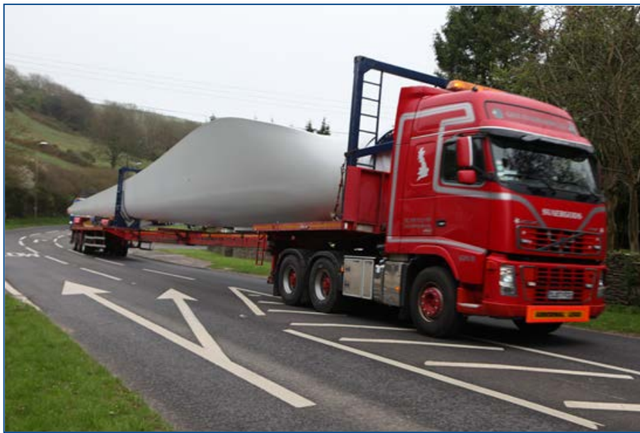
Figure 16.3: Typical Delivery of Wind Turbine Blade
